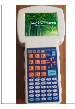
Digi-PDA (Personal Digital Assistant) is especially designed for industrial applications that may vary from one need to another. It's built on the Modulus platform, so it's easily extended using a wide range of hardware modules - anything from passport readers and fingerprint WAN radios, scanners to scanners, imagers and Bluetooth® printers. Plus a growing range of connectivity peripherals (RS232, USB...) that mean you'll never regret your decision.
